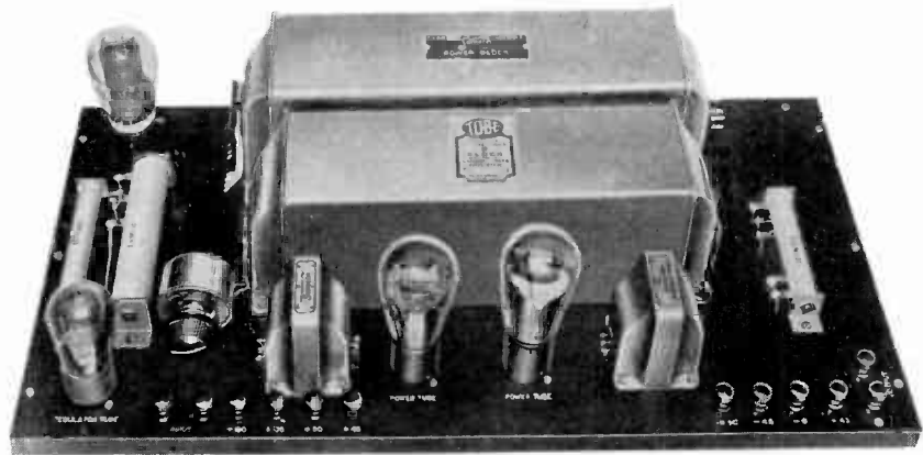
The completed Samson De Luxe Power Amplifier which employs a 210 push-pull unit as the output stage.
